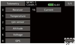
If you do not want to display telemetry data on the telemetry monitor screen, select "---".
