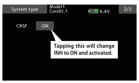
2 Tap the "CRSF" button to [ON]. A signal conforming to the CRSF standard is output from the S.BUS setting connector (S.I/F) of the transmitter.
