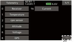
If you do not want to display telemetry data on the telemetry monitor screen, select "---".
