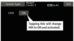
② Tap the "CRSF" button to [ON]. A signal conforming to the CRSF standard is output from the S.BUS setting connector (S.I/F) of the transmitter. Futaba is not responsible for damage sustained by combination with parts other than Futaba Genuine equipment.
